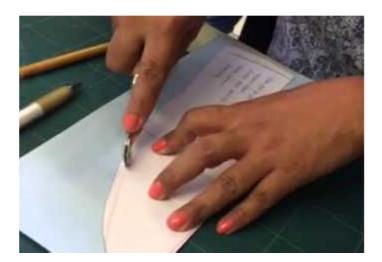
Once cut all the pieces, the vast majority must carry a series of figurative pen, and these figurados guidelines that will use the aparadora to assemble the pieces together. This pen ink disappear easily rub.
