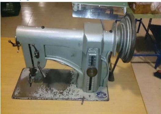
It is a machine that, as its name implies, itches around the bottom of the shoe (the one that comes in contact with the sole) in order to carry the corresponding holes and facilitate sewing by "point of buttonhole".
