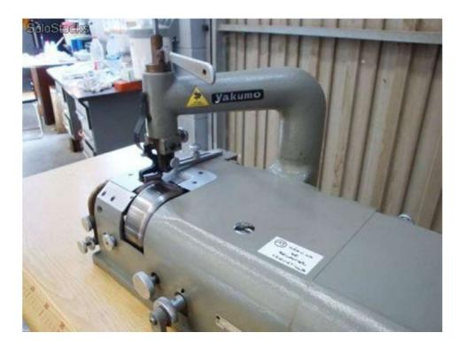
It is used to reduce the thickness at the edges of the pieces. Its purpose is:
